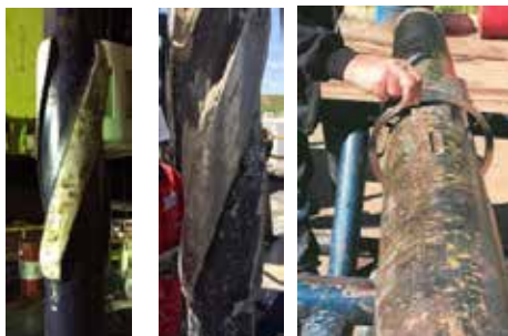
Figure 2. Surface of the stabilizer before and after the field tests at TPAO Beşikli-34 well.
