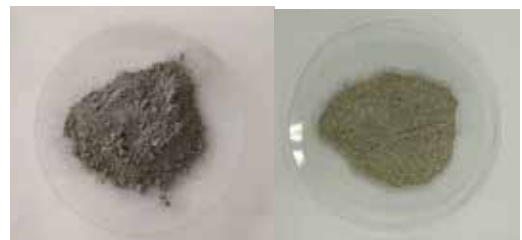
Figure 4. Raw and calcinated aluminium white dross at 1000°C
