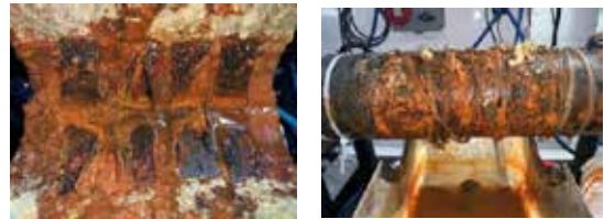
Figure 3. Coupons(left) and pipe(right) inside CUI test rig
