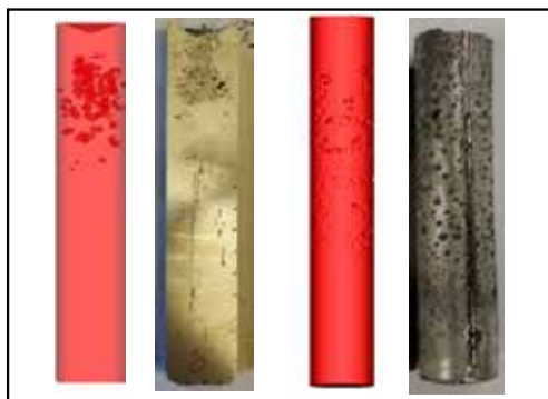
Figure 8. Validation of parameter set and a comparison of the surface porosity with refined mesh.
