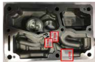
Figure 4. Shrinkage porosity regions on the part
