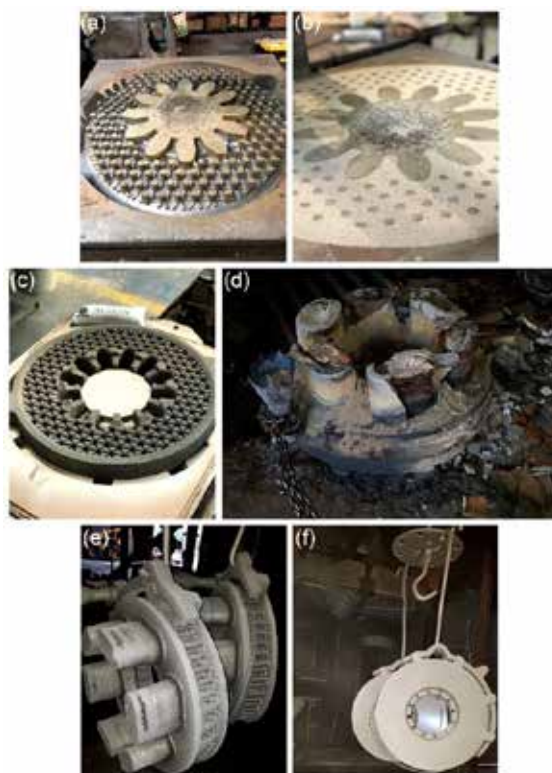
Figure 2. Casting trials of 4140 alloy high-speed train's brake disc (a), (b) core, and (c) mold preparation (d) shakeout (e) casting is ready for shot blasting and (f) after shot blasting
