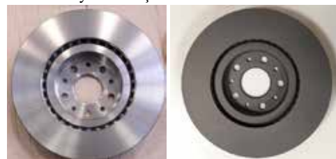
Fig 1. Brake discs: Untreated (left), FNC treated (right) disc.
