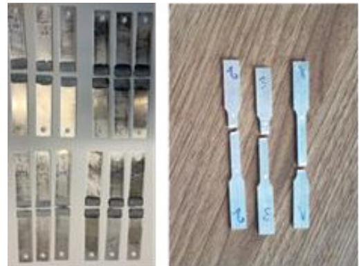
Figure 4 Raw material and adhesive lap joints test specimens after tensile tests
