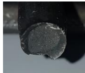
Figure 2. Ductile Fracture Surface (15,0 mm C82D)
