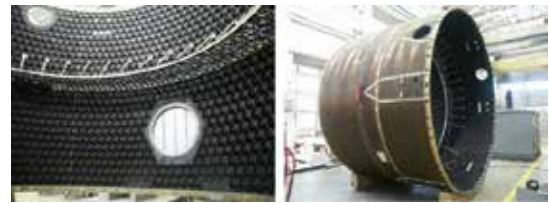
Figure 4. Internal (left) and external (right) view of the upper interstage of Proton M Launcher [11]
