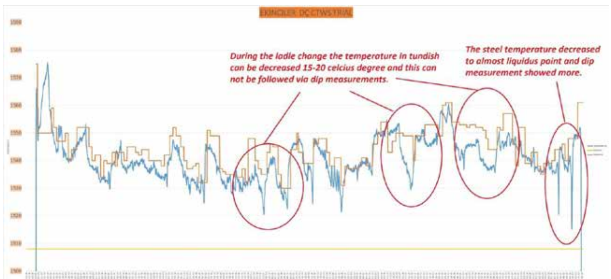
Figure 3: The temperature traces during one tundish sequence. Blue lines (Castemp) - Orange lines(Dip measurements)
