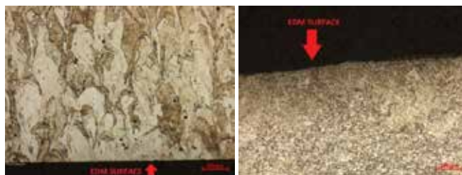
Figure 1. Microstructure of a) as-built and b) solution heat treated specimen after EDM cutting.
