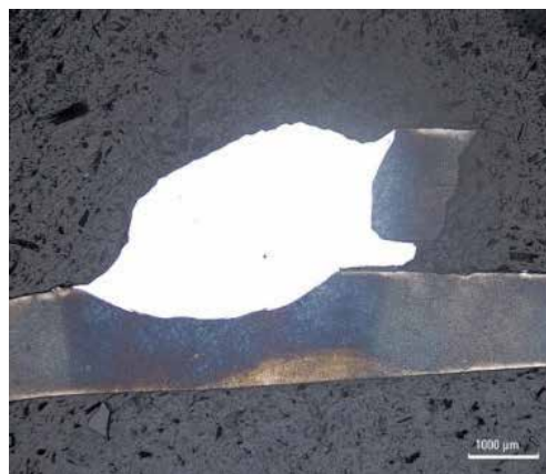
Figure 6. Fractured sample of weldment with speed of 150cm.min -1
