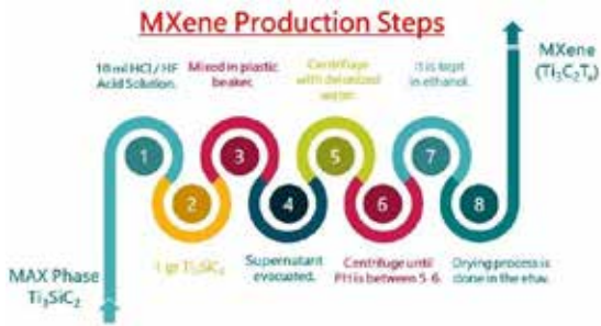
Figure 1: Production Phases from MAX Phase to MXene.
