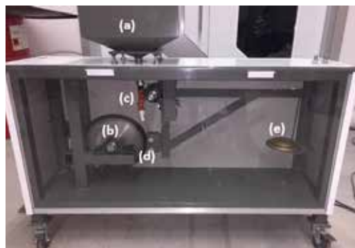
Figure 1. Abrasion Test Unit (ASTM G65 Standard), (a) Sand Unit, (b) Rubber Wheel and Rotary Drum, (c) Sand Sprayer, (d) Test Sample, (e) Weight [14]
