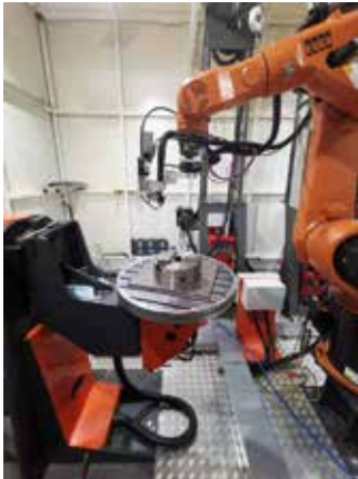
Figure 1. Experimental WAAM system: an industrial robot and a two-axis positioner.
