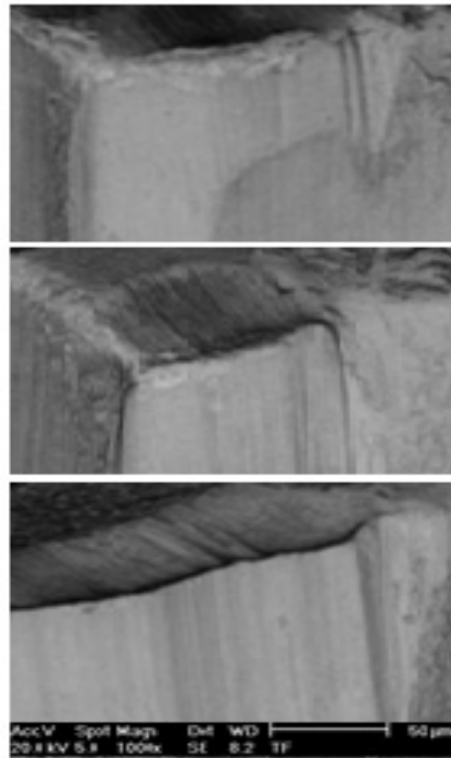
Figure 1. Wear patterns of PCBN tools in continuous milling
