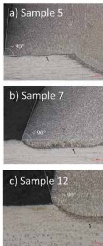
Figure 4 Bead-substrate interface of samples (a) 5, (b) 7 and (c) 12
