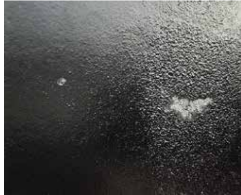
Figure 2. Macro image of enamel surface of cast iron specimen (Left side of specimen was sandblasted at 3 Bar for 2.5 min. Right side of specimen was left untreated).
