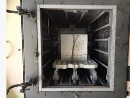
Figure 1. Placement of the NADCA test specimen in the furnace.
