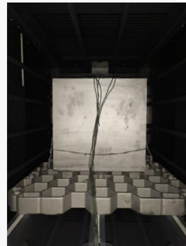
Figure 5. Test block after NADCA test.
