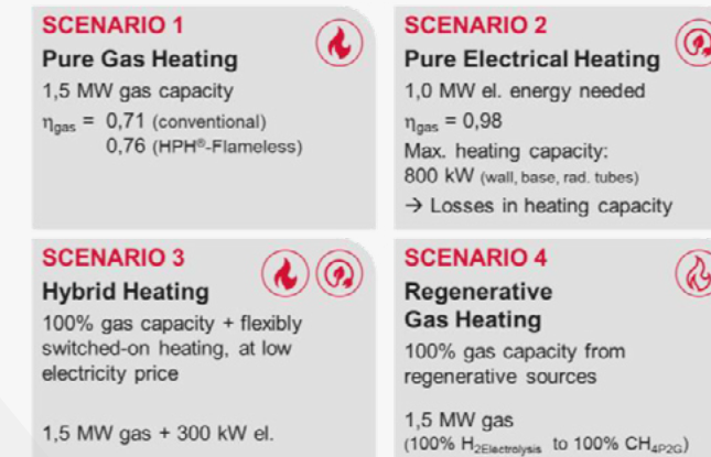
Figure 3. Overview of scenarios for decarbonisation of the bell-type annealing process.
