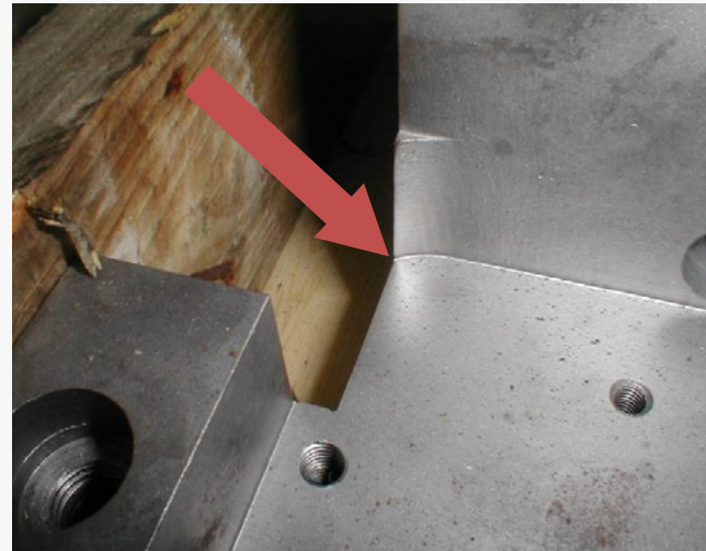
Figure 13. Narrow radius in a HPDC die
