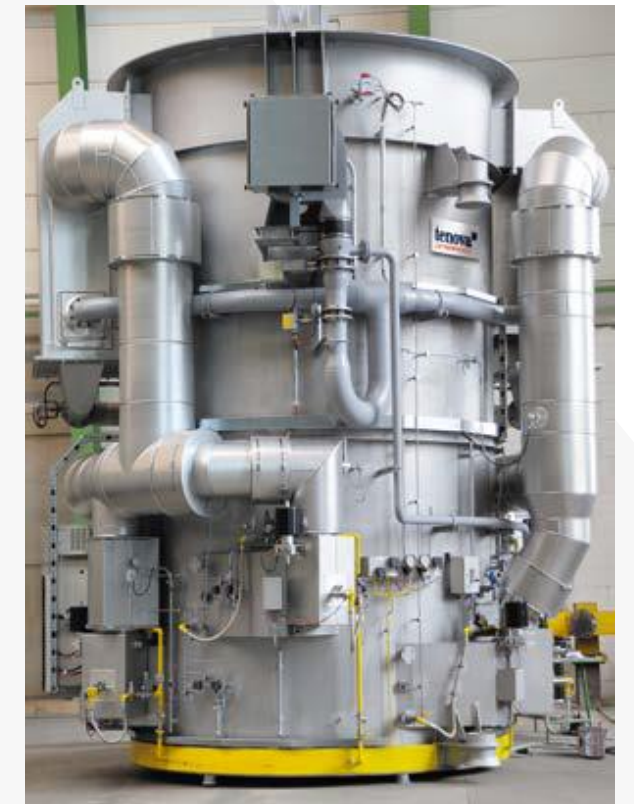
Figure 4. Tenova LOI Thermprocess Ultra-low NO x HPH ® -flameless heating hood.
